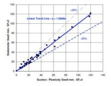
Comparing strains ('y' axis) with suctions ('x' axis) reveals a good correlation, improving as the soil becomes increasingly desiccated. A shrinkage factor of 2 has been used for the oedometer, and 4 for suctions.
