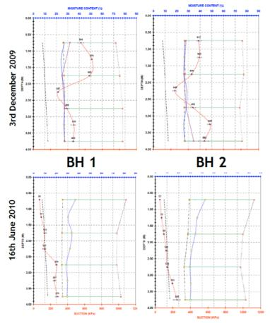
Boreholes sunk in front of the two damaged bay windows. The first investigations were undertaken in December 2009 and the second (bottom) in the middle of July, 2010.
